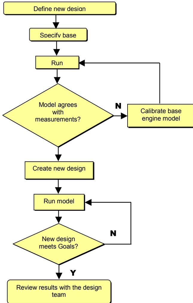
Fig 1: Traditional Simulation-based Design Process
