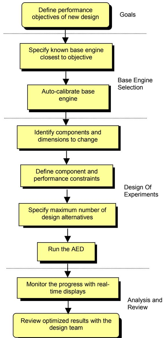
Fig 2: Simulation-based Automated Design process
